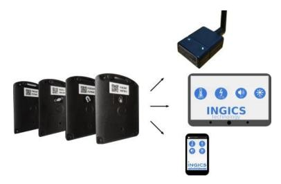
2. Use iGS01 beacon gateway to receive the beacon message and send to cloud server. You can then access and manage the data anytime anywhere.
