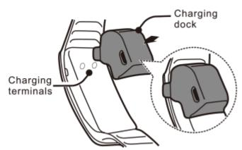
Make sure the charging dock is connected with device closely and the USB cable is in good
