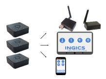
2. Use iGS01S or iGS02E beacon gateway to receive the beacon message and send to cloud server. User can access and manage the data anytime anywhere.
